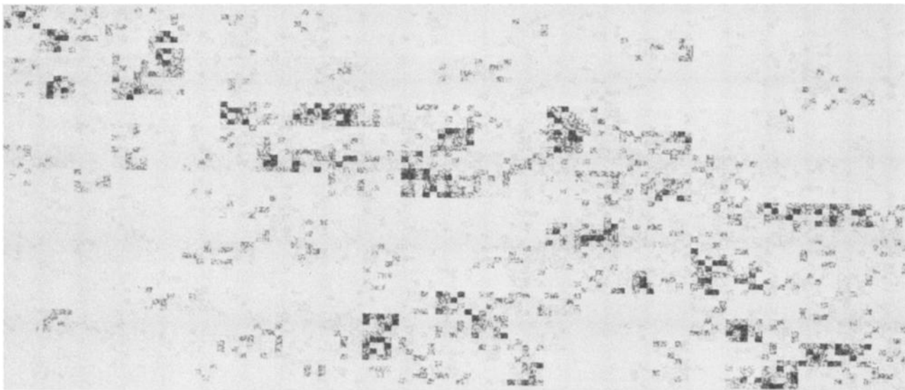
Fig. 4. An example of a (random) anisotropic \alpha -model with d_s = \log 20 / \log 5 = 1.86 , C(1) = 0.16 , C_\infty = 0.46 , with grey shades proportional to the log of \varepsilon .
