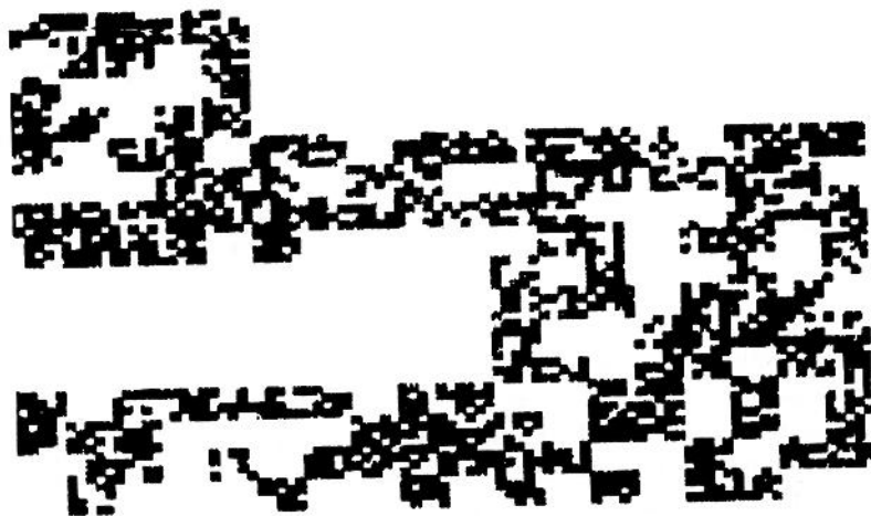
Fig. 8. A random curdling on an anisotropic grid, with D_{cl} = \log 20 / \log 5 = 1.86 \dots . All eddies are either "dead" or "active", such that the dimension of the support is: D_s = 1.70
