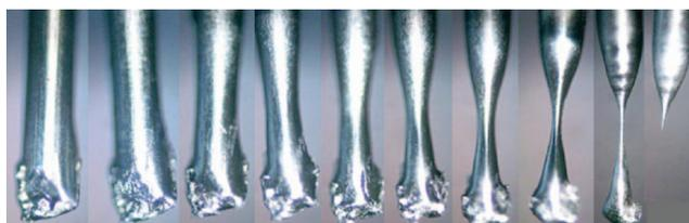
FIG. 1. (Color online) 0.25 mm Ir wire during the coarse etching at roughly 30 s intervals.
